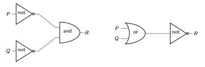
Figure: Two equivalent digital circuits
