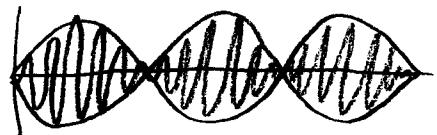
$$\text{Case 1: } w \neq w_0. \quad x(t) = \frac{A}{w_0^2 - w^2} (\cos wt - \cos w_0 t) = \frac{A}{2\delta\bar{\omega}} \sin \delta t \sin \bar{\omega}t$$
