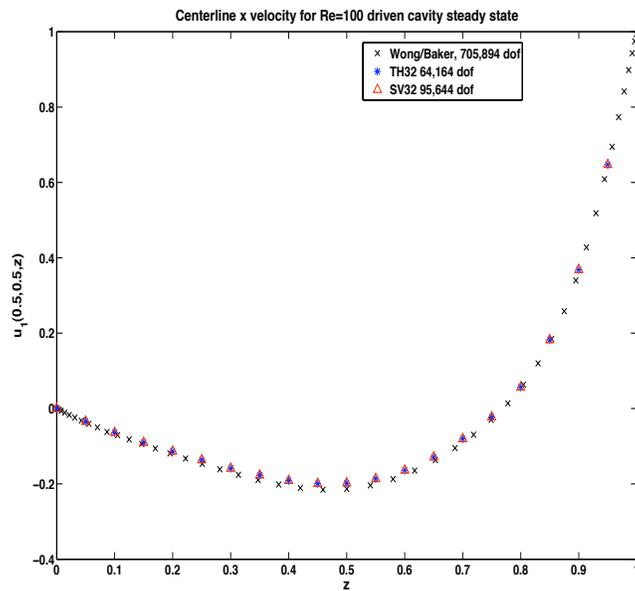
Figure 2.13: 3D lid-driven cavity results compared to “true” solution on centerline.
