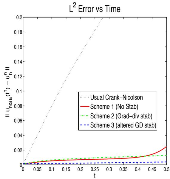
Figure 3.2: The plot above shows  $L_2$  error of the velocity vs time for the four schemes of Test 2. We see in the plot that the stabilizations add accuracy to the enhanced-physics scheme, and that the alternate grad-div stabilization gives slightly better results than the usual grad-div stabilization. It can also be seen that the enhanced-physics scheme is far more accurate in this metric than the usual CCN scheme.
