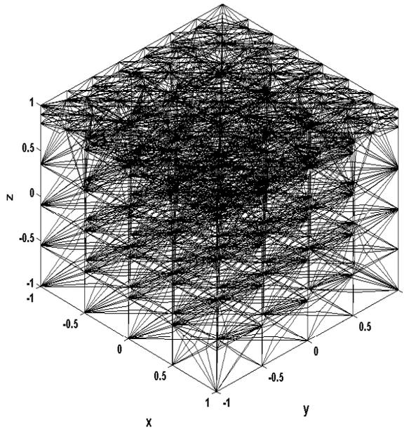
Figure 2.10: The barycenter-refined mesh used for the 3D lid-driven cavity problem.
