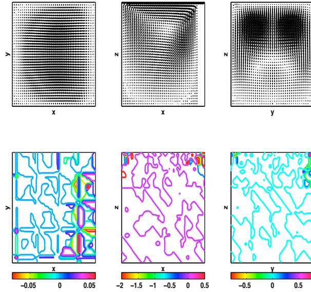
Figure 2.12: 3D lid-driven cavity results with TH elements. Note the scale next to the color bar and the contours in the corners of each midplane.
