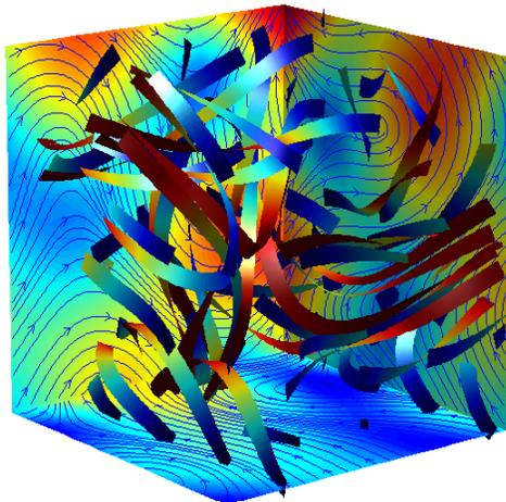
Figure 3.1: The velocity solution to the Ethier-Steinman problem with  $a = 1.25$ ,  $d = 1$  at  $t = 0$  on the  $(-1, 1)^3$  domain. The complex flow structure is seen in the streamribbons in the box and the velocity streamlines and speed contours on the sides.
