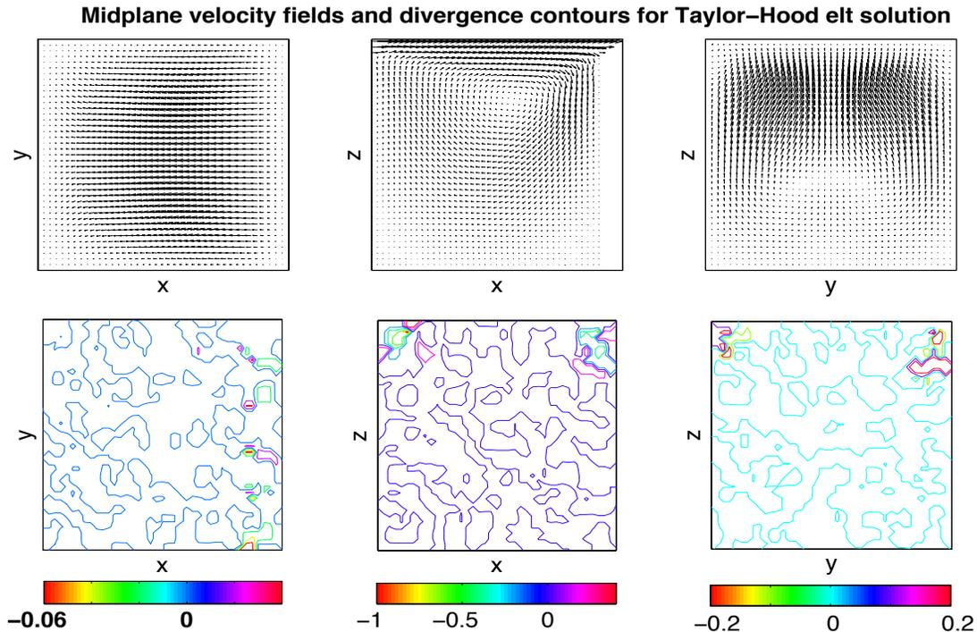
Figure 4.5: For TH with  $\gamma = 0$ , we see the expected velocity profiles for the lid-driven cavity problem, with non-negligible error for  $\text{div } \mathbf{u}_h$ .
