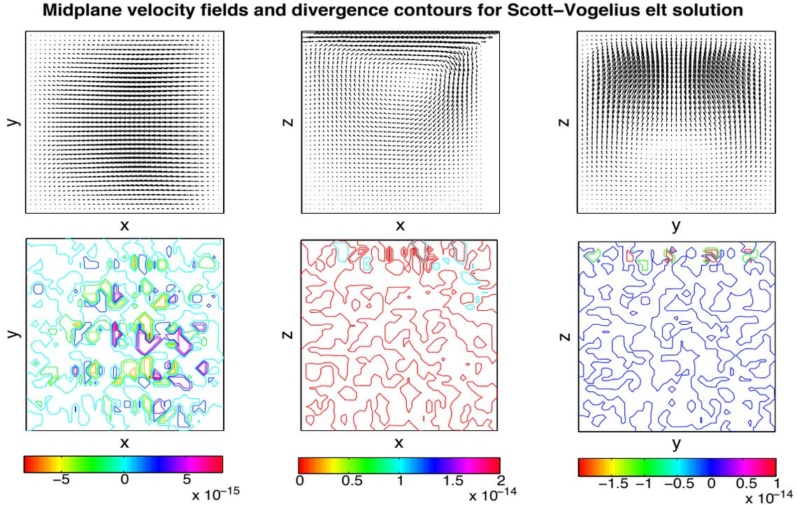
Figure 4.4: We see the expected velocity profiles for the lid-driven cavity problem with  $\text{div } \mathbf{u}_h$  close to machine epsilon.
