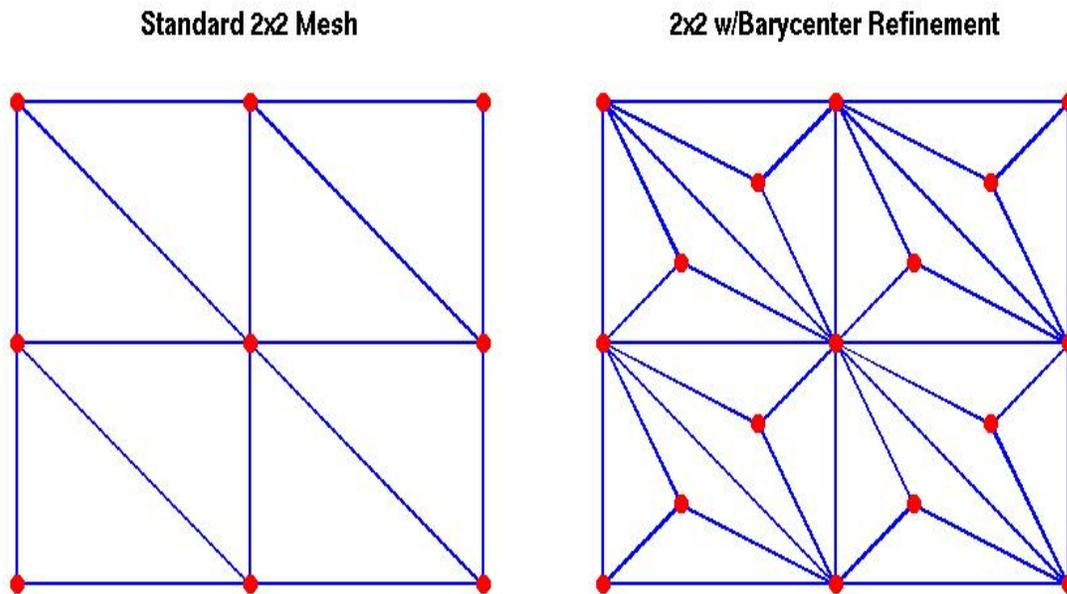
Figure 2.2: (LEFT) 2D conforming mesh and (RIGHT) mesh resulting from barycentric refinement.
